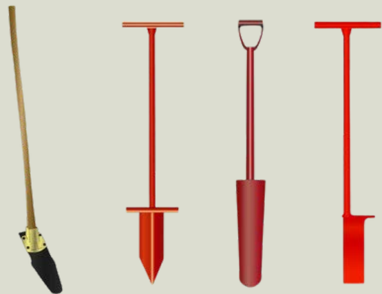
Four common tree-planting tools from left to right: Hoedad, KBC planting bar, sharpshooter spade, and dibble bar.
