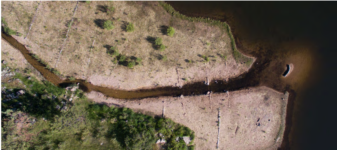
Top: Aerial showing sediment delta formed from post-fire erosion with some post-restoration structures visible. Bottom, left to right: Volunteers installing erosion control structures; crews stabilizing channel.
